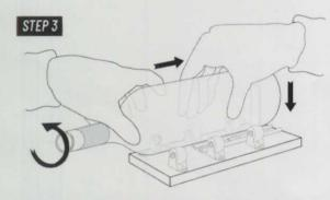
Apply just enough downward pressure on the bottle so that it scores a line in the glass. Make sure to hold the bottle down towards the back brace at all times to keep a straight cut.
