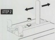
Adjust the back brace so that it touches the bottom of the bottle. Tighten the screw again to hold it back in place.
