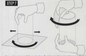
Use sandpaper to smooth the rough edges. To make even edge, put sandpaper on table and sand the top edge. Then sand the inner and outer corners of the glass edge by hand.
