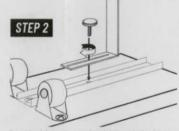
Insert back brace into track and tighten the knob screw
