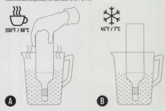
Heat up the score line. Dip the bottle into a tub or container of hot water and then switch to cold water, and make sure the water covers the cut.
