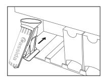
Figure 3 - Installing coin tube
