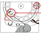
COIN PRESENCE SENSOR: (Intensify spraying under the sensor) 12. Reinstall the housing. Housing must be properly lined up with the AC power cord and power switch at the back of the machine. Do not force the housing while placing it back, as this could damage the coin feed mechanism built into the housing.
