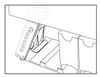
Figure 4 - Coin tube in proper position
