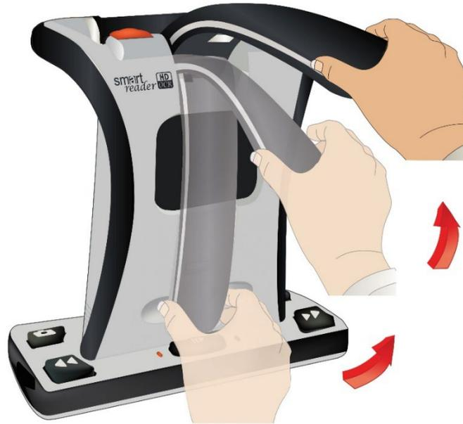
1. Depressions are on the Smart Reader body behind each side of the camera arm. Use these depressions as guides for gently gripping both sides of the arm.
