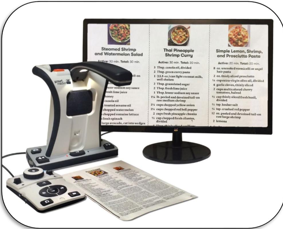
With display mode, an external display such as a television or computer monitor is connected to the HDMI port on the back of the device.
