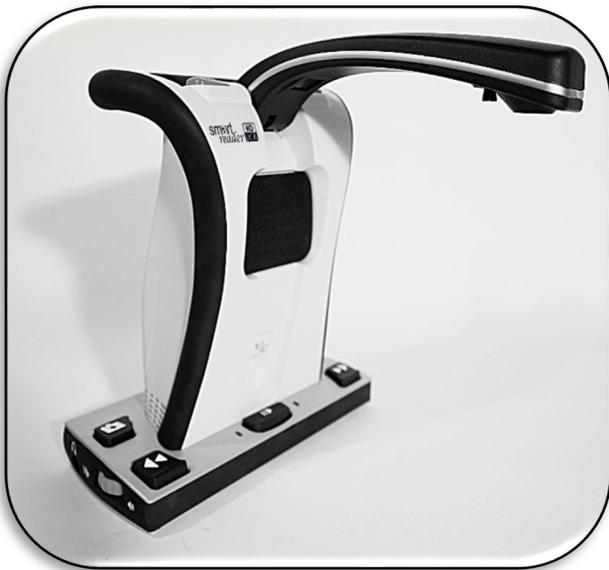
With standalone, no display device is connected to the base unit. The menu and annunciations are optimized to be fully navigable through sound. After scanning a document, the OCR results are played back as speech through the front speaker in the base of the unit. Some features with strictly visual utility such as color mode adjustments are filtered out for users who do not have a visual display.
