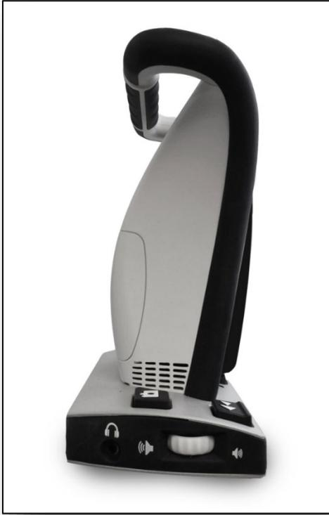
2. Carry Smart Reader HD only by the handle on the back of the unit for a secure grip. Gently place it on the table or desk.
