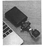
Power bank to be tested should be fully charged, then plug multimeter and reset power time by long pressing, connect phone or load or other discharging devices. Until power banks completely discharged by the multimeter, its power capacity will be tested and multimeter will read the data when electrifying again.
